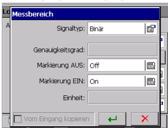
The screenshot shows the 'Messbereich' (Measurement Range) configuration window. The 'Signaltyp' (Signal Type) is set to 'Binär' (Binary). Other fields include 'Genauigkeitsgrad' (Accuracy), 'Markierung AUS' (Off), 'Markierung EIN' (On), and 'Einheit' (Unit). A checkbox at the bottom is labeled 'Vom Eingang kopieren' (Copy from input).
